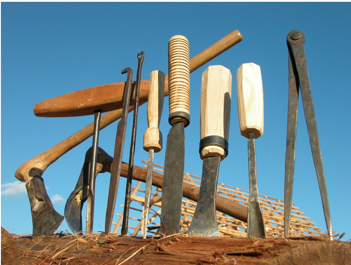
Fig. 2: Different types of woodworking tools, the use of which could be proven at the Dürrenberg: from left to right: heavy grommet axe and flap axe on knee wood shafts, spoon drill, carving knife, bark sewing needle, scribing awl, pull saw, chisel, gouge and compass (Photo: Wolfgang F. A. Lobisser).
